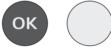
If the indicator of temperature turns **WHITE**, this means that the temperature is too high; in this case, increase the refrigerator temperature control setting and wait for 12 hours before performing a new visual inspection of the indicator.
