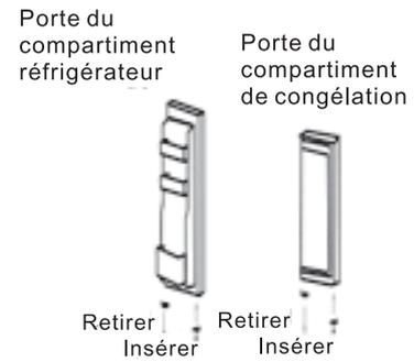
6. Place the fridge door on the lower hinge, making sure that the hinge pin is inserted in the hole at the bottom of the fridge door. Put the middle hinge back on the cabinet, making sure that it is on the opposite side from its original position.
