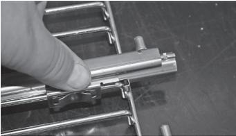
Mounting Suggestions; side wire racks have to be completely dismantled from the oven, than mount the rails on to the side wire racks on a flat surface. Please mount the telescopic rails to the above wire on the shelf. The rails can be easily mounted and dismantled. After arranging the positions of the right and left telescopic rails, push them until the fixing clips are fully mounted on the shelf wire.
