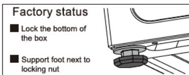
⚠ **Note:** In order to facilitate installation, the factory status of the foot may not be all locked, please be sure to lock all four feet before adjusting the level
