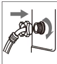
2. Connect the other end of the inlet hose to the inlet valve at the backside of the washing machine and fasten the hose tightly clockwise. when there is a inlet at the back of the machine, it must be connected to a cold water supply.
