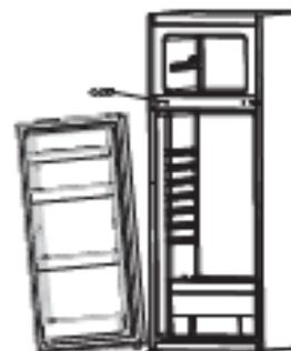
7. Place the fridge door on the middle hinge, making sure that the hinge pin is inserted in the hole at the bottom of the fridge door. Then put on the upper hinge, aim at the door and screw down the bolt, cover the left hinge cover and then screw down the bolt.
