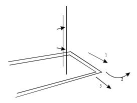
According to the needs of food storage, you can adjust the shelf to proper position; To facilitate the use of it or adjustment the location, the shelf can be set to slip so that you can use and adjust it easily when you want to clear the shelf, please move the shelf by the direction(1), then turn the shelf in the direction(2) for 90° until it is Perpendicular to the original direction, pull out the shelf by the direction (3).
