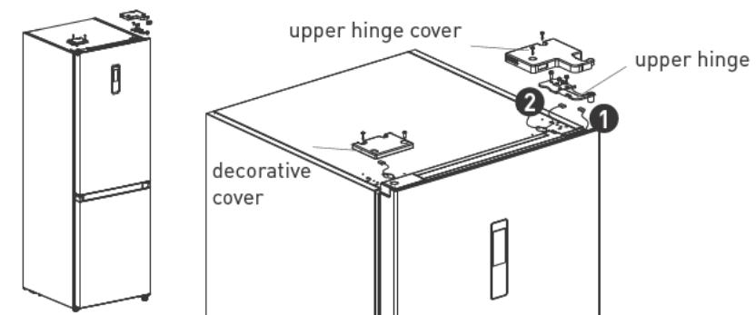
3. Remove the refrigerated door body (be careful not to lose small parts such as the shaft sleeve and stop on the door);
