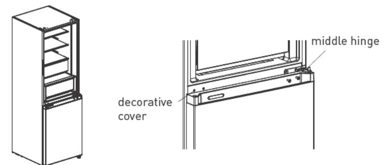
4. Remove the freezing door body (be careful not to lose small parts such as the shaft sleeve and stop on the door);
