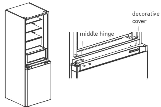
8. Remove the upper left hinge cover and upper left hinge from the accessory bag. Place the refrigerated door body on the middle hinge and install the upper left hinge. Connect the refrigerator top signal line ④ to the door body signal line ①, and connect the signal line ② to the signal line ③. Finally, replace the hinge decorative cover to the right side of the box body.
