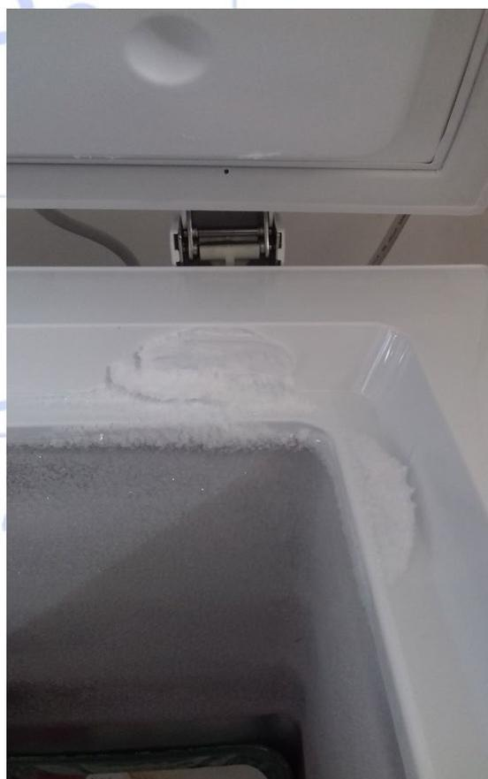
In order to facilitate the opening of the cover, the seal is perforated at the level of the hinges. This may result in a small formation of frost on the case or the lid of the product. **This frost is completely normal and must be removed regularly so as not to interfere with closing the lid.**
