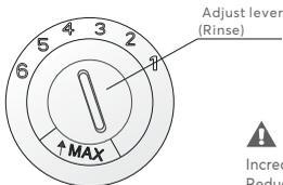
The rinse aid dispenser has six or four settings. Always start with the dispenser set on "4". If spots and poor drying are a problem, increase the amount of rinse aid dispensed by removing the dispenser lid and rotating the dial to "5". If the dishes still are not drying properly or are spotted, adjust the dial to the next higher number until your dishes are spot-free. The recommended setting is "4". (Factory value is "4".)
