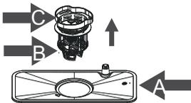
Step 2: Lift B and C up from A;
