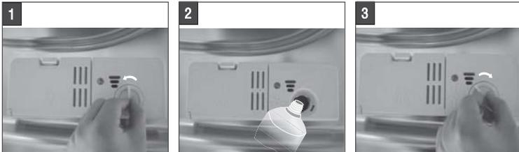
1. To open the dispenser, turn the cap to the "open" (left) arrow and lift it out.
