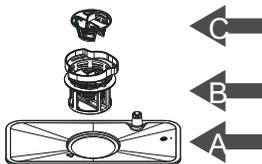
Step 3: Separate B and C.
