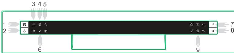
1. Power Button: To turn on/off the power supply.
