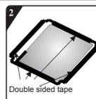
Remove surface paper on double sided tape at four sides of the bottom plate.
