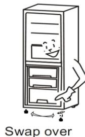
5. Remove the hinge pin that is in the bottom of the fridge and freezer door. At the other side of the fridge and freezer door, insert the replacement hinge pin that is supplied with the appliance.
