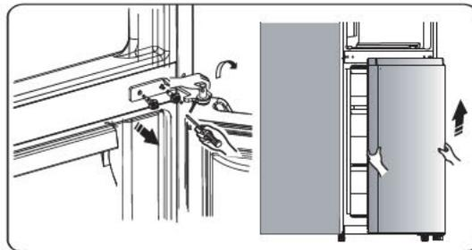
7. Place the lower door on a smooth surface with its panel upwards. Use a putty knife or thin-blade screwdriver to prize part1, then install it to the opposite side and tighten it securely.
