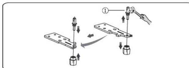
11. Replace the lower hinge part to the left side and fixing it with the special flange self-tapping screws. Replace the adjustable bottom feet parts to another side and fixing it.
