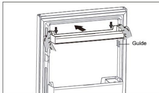
Firstly hold the two side of the door shelf tightly, fit the door shelf along the guides on the door, then push it down to the right place.
