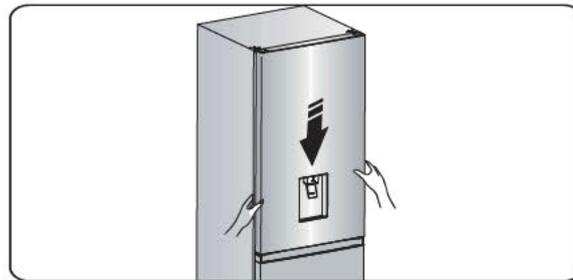
15. Move the upper door to an appropriate position, and then fix part 4 by screws 3. (Please hold the upper door by hand when installing). Install the upper hinge cover 2 on the left corner by screw 1.
