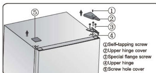
3. Remove the upper door from the middle hinge by carefully lifting the door straight up.
