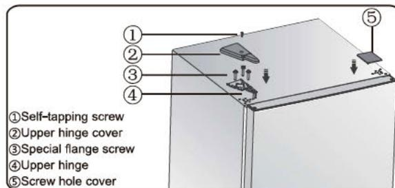
16. Install the screw hole cover<sup>5</sup> on the top right corner of the refrigerator.
