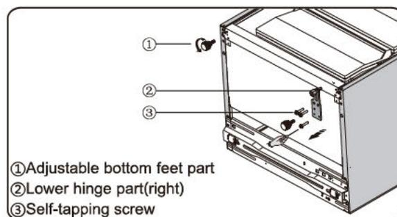
10.Remove part 1 from the lower hinge part(right), loose out the lower hinge pin, change it to the reverse hole site, and then tighten into position, then install part 1 on the lower hinge pin.
