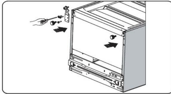
12. Transfer the lower door to the property position, adjust the lower hinge part, make the hinge axis into the lower hole of the lower door, then tight the bolts.
