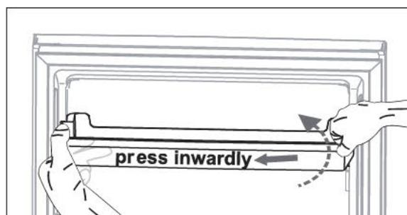
Hold one side of the door shelf, press the opposite side inwardly by the other hand, then lift up the door rack . When the slot of the door rack has been detached from the guide on the door, remove the rack upward obliquely.
