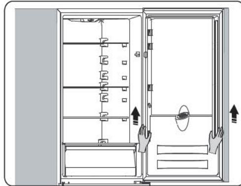
4. Place the upper door on a smooth surface with its upper cover upwards.
