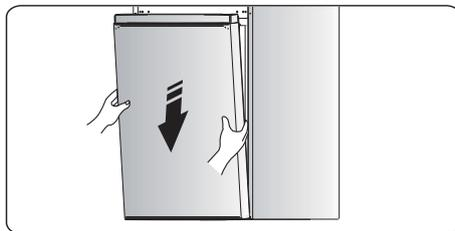
13. Slot the lower door onto the bottom hinge pin and hold in position. Turn the middle hinge by 180°, change the washer on the axis to the lower side, adjust the middle hinge to the appropriate position and then install it ensuring the lower door is secured in place.
