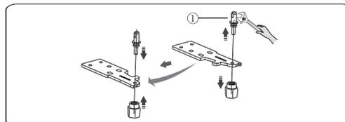
11. Replace the lower hinge part to the left side and fix it with the special flange self-tapping screws. Replace the adjustable bottom feet parts to another side and fix it.
