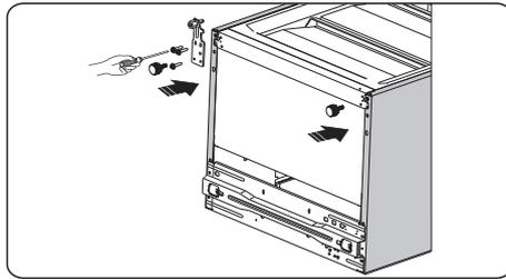
12. Transfer the lower door to the proper position, adjust the lower hinge part, make the hinge axis into the lower hole of the lower door, then tighten the bolts.
