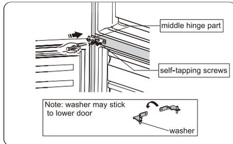
14. Transfer the upper door to the appropriate position. Secure the door's level, make the middle hinge axis into the lower hole of the upper door.
