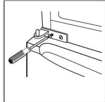
10. Place the upper door back on. Ensure the door is aligned horizontally and vertically so that the seal are closed on all sides before finally tightening the top hinge. Then insert the hinge and screw it to the top of the unit.
