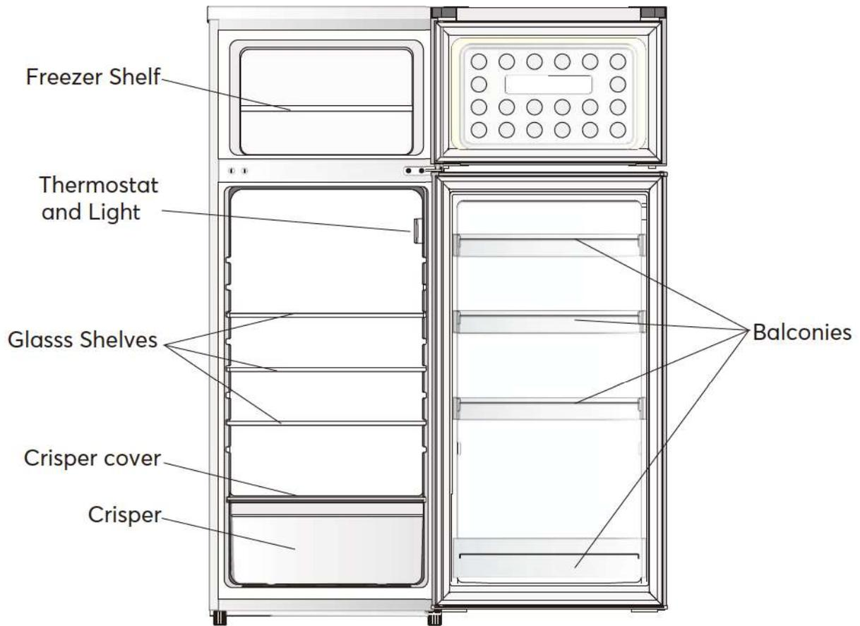
Drawers, food boxes, shelves, etc. placed according to the position in the picture above are the most energy efficient.
