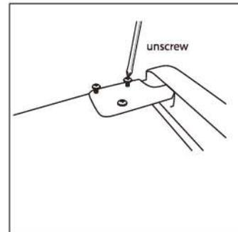
3. Remove the pin with a screwdriver and flip the hinge bracket. Then refit the pin to hinge bracket.
