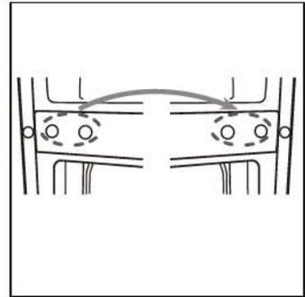
6. Unscrew bottom hinge. Then remove the adjustable feet from both side.
