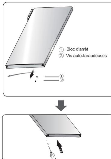
6. Lay the refrigerator on soft foam packaging or similar material. Remove both adjustable bottom feet parts, and the lower hinge part by unscrewing the special flange selftapping screws.
