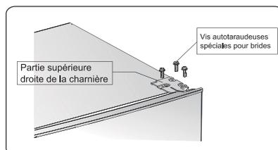
3. Remove the upper hinge axis, transfer it to reversed side and tighten securely, then put it in a safe place.
