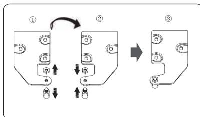
4. Remove the door from the lower hinge.
