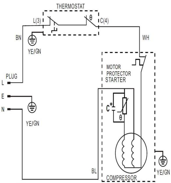
**C\***:The capacitor is optional according to different compressor model
