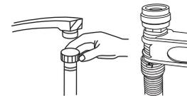
Connect the straight connector of the inlet hose to the water supply securely ensuring that the washers are securely in place at both ends of the hose.
