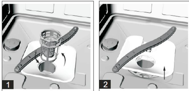
Turn the assembled central and micro filters anticlockwise to unlock them from the appliance.
