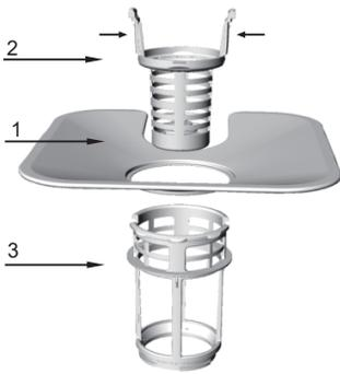
The filter system consists of a coarse filter, a flat (Main filter) and a micro filter (fine filter).
