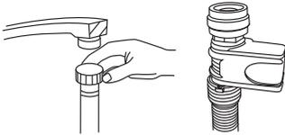
Connect the cold water supply hose to a threaded 3/4(inch) connector and make sure that it is fastened tightly in place. If the water pipes are new or have not been used for an extended period of time, let the water run to make sure that the water is clear and free of impurities. If this precaution is not taken, there is a risk that the water inlet can get blocked and the appliance could be damaged.
