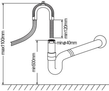
Fit the drainage hose of your machine to the drainage pipe without bending.
