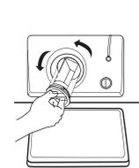
4. Open the filter by turning to the counter clockwise
