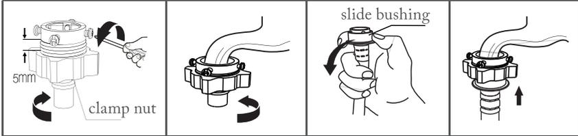
Loosen clamp nut and four bolts
