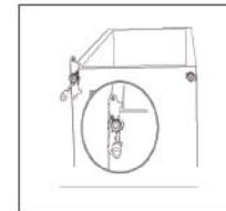
7. Place the upper door back on. Ensure the door is aligned horizontally and vertically so that the seals are closed on all sides before finally tightening the top hinge.
