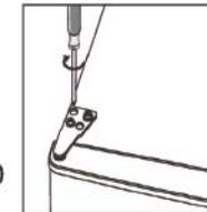
8. Insert the hinge bracket and screw it to the top of the unit.
