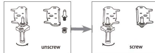
6. Refit the bracket fitting the bottom hinge pin. Replace both adjustable feet.
