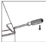
2. Undo the screws. Then remove the hinge bracket.
