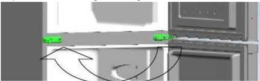
8. Position the the bottom door in place and fix the middle hinge.
