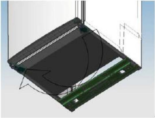
6. Transfer the levelling foot to other side and adjust it unit it is level.
