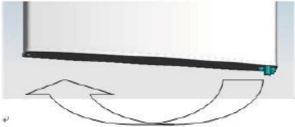
5. Reposition the bottom hinge to the other side then fix it with screws.
