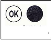
If "OK" is not displayed, the average temperature in this area will be very high. You ought to adjust the thermostat to a colder setting.
