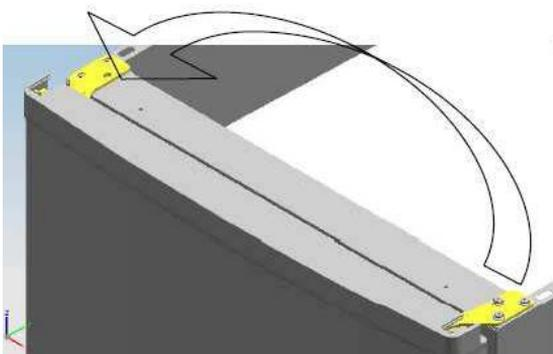
10. Position the top door in place and fix the top hinge then attach the cover.
