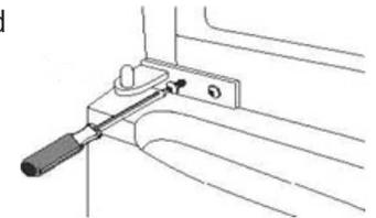
4. Remove the door stop of the Freezer door and put it to the opposite side. Align the lower hole of the door to the gun of the left middle hinge while taking care of the alignment of the door compared to the refrigerator.
