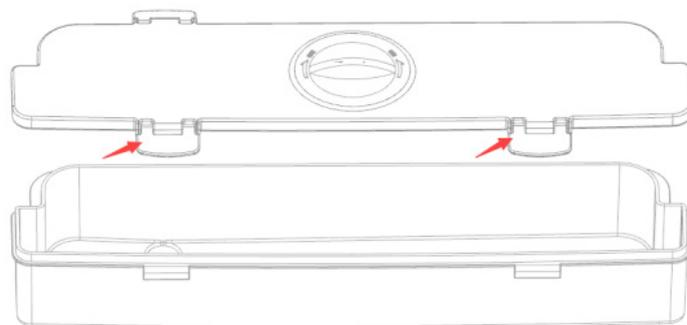
4. Disassemble the parts, clean the interior and exterior of the tank with a clean sponge or soft cloth, use warm water or 1 teaspoon of bicarbonate of soda dissolved in 1.2 liters of water.
