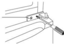
5. Then unscrew the front foot to remove the bottom hinge.
