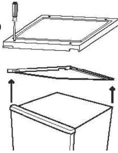
2. Remove the left hinge cover. Insert the right hinge cover.
