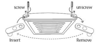
3. Position the middle hinge on the left of the refrigerator and insert the gun of hinge in the hole of the door then fix it firmly.
