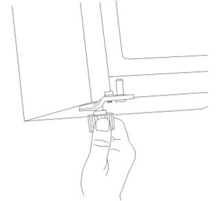
2. Remove door stopper from the fridge door and put it to the opposite side. Align the hole of the door to the gun of the hinge while taking care of the alignment of the door compared to the refrigerator.
