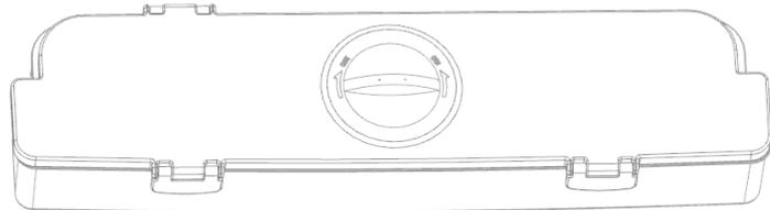
2. Remove upward the water tank from refrigerator door.
