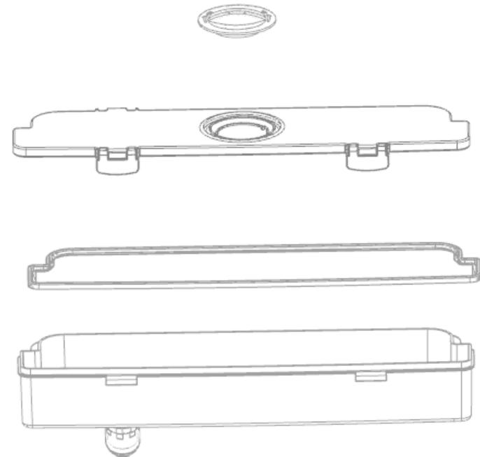
5. Install dispenser in reverse steps and fix the water tank back to the door.
