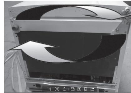
5. Reinstall the door on the hinge properly, take care about the vertical alignment
