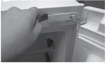
2. Unscrew and remove the hinge with a cross-slot screwdriver
