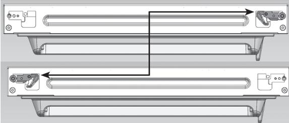
c. Use a tool to remove the axle and two stoppers on the lower hinge and then assemble them to the position as shown in the below figure.
