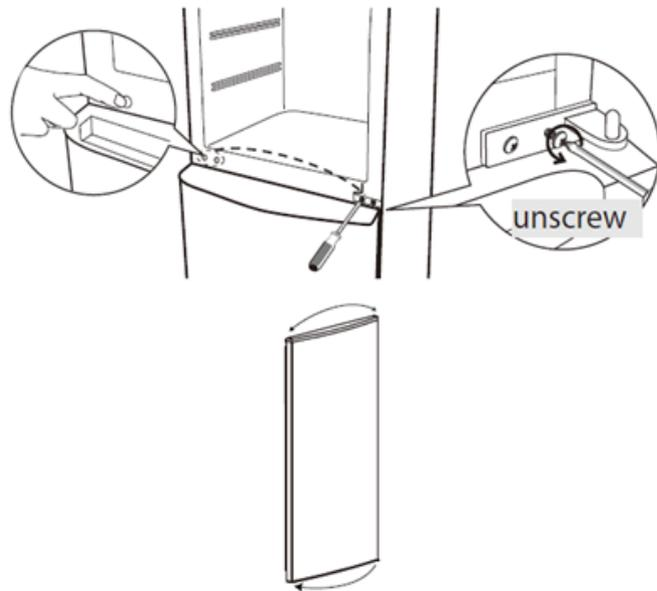
4. Remove the lower screws and lower hinge from the unit bottom. Reverse the lower hinge, move and secure it with the lower screws to the opposite side of the unit bottom. Carefully set the lower door back into place, inserting it onto the lower hinge.
