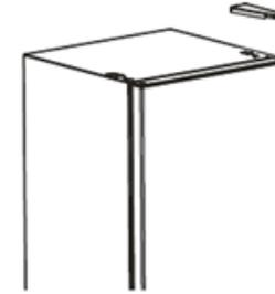
2. Remove the the upper hinge. Lift the upper door and place it on a padded surface to prevent it from scratching. Remove the door block, screw and plastic tube under the upper door and move them to the opposite side. You may need to replace the door block to fit the opposite side.
