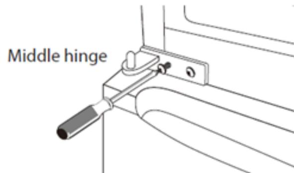
6. Carefully set the upper door back into place, inserting it onto the middle hinge.
