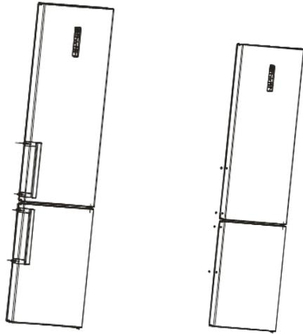
4. Install the handles into the door handle holes of the other side in accordance with the handle installation instructions.
