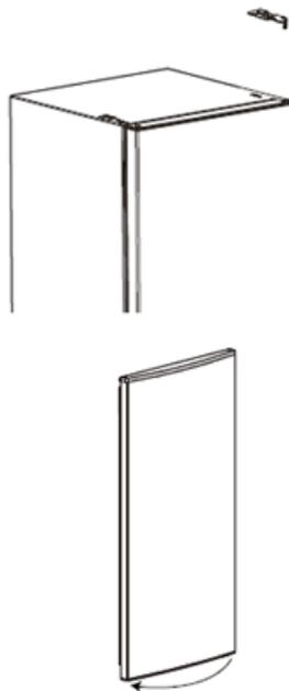
3. Take off the middle hinge by removing the screws. Lift the lower door and place it on a padded surface to prevent it from scratching.
