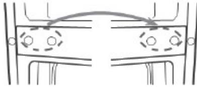
7. Unscrew bottom hinge. Then remove the adjustable feet from both side.
