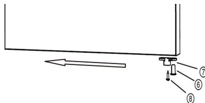
4. Dismantle the levelling foot ⑩, positioning bolts ④ and lower hinge ⑨, then exchange the parts of right and left sides and later use the reverse method to install the levelling foot and positioning bolts.
