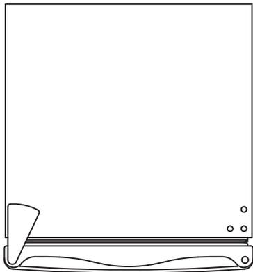
4. Put on the door to bottom hinge, then fix top hinge and cover.
