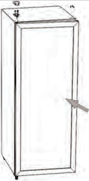
5. Align the lower hinge axle hole into the door body. Install the door hinge and 3 screw covers on the other side.
