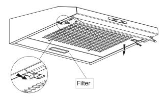
The efficiency of the hood is conditioned by the cleanliness of the air inlet and of the filter.
