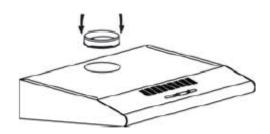
7. Open the grease filter, secure the hood with the 2 screws provided. (Maximum length of 30 MM)
