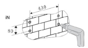
3. Insert dowels (not supplied) into the holes corresponding to the type of material of your wall.
