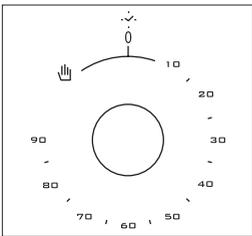
**Mechanical timer\*:** Used for determining the period for cooking in the oven. When adjusted time is expired, power to heaters is turned off and an audible warnig signal is emitted. Mechanical timer can be adjusted to desired period between 0-90 minutes. For cooking periods, see cooking tables.
