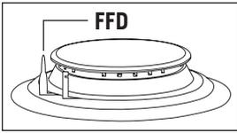
**Flame cut-off safety device (FFD) \***; operates instantly when safety mechanism activates due to overflow liquid over upper hobs.
