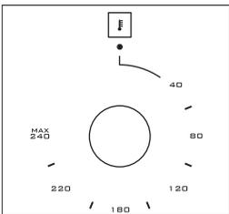
**Thermostat:** Used for determining the cooking temperature of the dish to be cooked in the oven. After placing the food inside the oven, turn the switch to adjust desired temperature setting between 40-240 °C. For cooking temperatures of different food, see cooking table.
