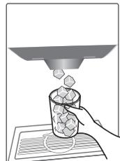
Touch “ GLACE PILÉE ” button; if
