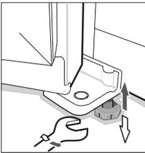
When the refrigerator stays in the packing box, plastic feet are in tightened state. After carrying it out from the packing box for placement, please make sure to adjust two front plastic feet until the height is suitable; just adjust two plastic feet with a wrench or directly by hand.
