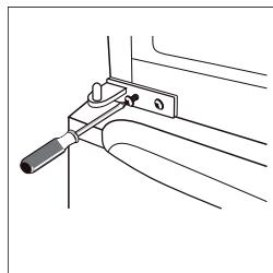
11. Place the upper door back on. Ensure the door is aligned horizontally and vertically so that the seal are closed on all sides before finally tightening the top hinge. Then inert the hinge and screw it to the top of the unit.
