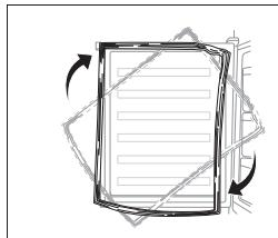
10. Make the middle hinge reverse the direction 180°C, then transfer it to the left property position. Make the middle hinge pin in the upper hole of the lower door, then tight the bolts.
