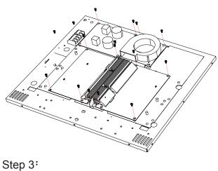
remove all the screws and wires
