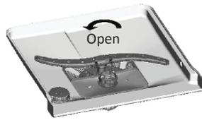
Step 1: Turn the filter in anti-clockwise direction,
