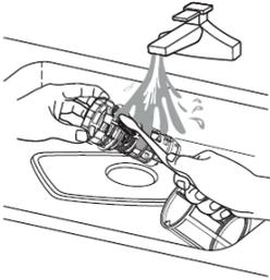
Larger food remnants can be cleaned by rinsing the filter under running water. For a more thorough clean, use a soft cleaning brush.
