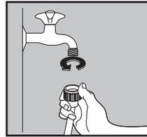
When there is an inlet valve at the back of the machine, it must be connected to a cold water supply. If there are two inlet valves, one is connected to a cold water supply and the other is connected to a hot water supply. Follow the indication of the picture below to complete the connection.
