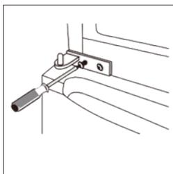
10. Place the upper door back on. Ensure the door is aligned horizontally and vertically so that the seal are closed on all sides before finally tightening the top hinge. Then inert the hinge and screw it to the top of the unit.
