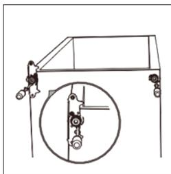
9. Make the middle hinge reverse the direction 180°, then transfer it to the left property position. Make the middle hinge pin in the upper hole of the lower door, then tight the bolts.
