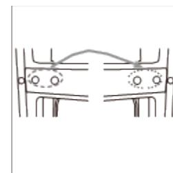
6. Unscrew bottom hinge. Then remove the adjustable feet from both sides.
