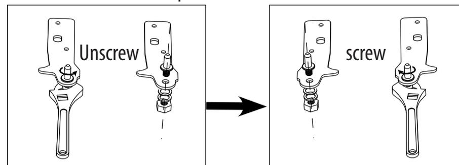
8. Refit the bracket fitting the bottom hinge pin. Replace both adjustable feet. Transfer the lower door to the property position.
