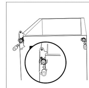
9. Make the middle hinge reverse the direction 180°C, then transfer it to the left property position. Make the middle hinge pin in the upper hole of the lower door, then tight the bolts.
