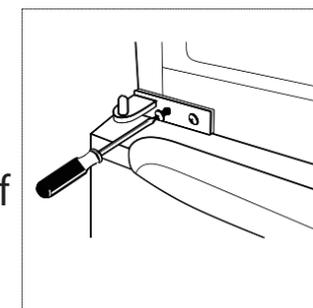
10. Place the upper door back on. Ensure the door is aligned horizontally and vertically so that the seal are closed on all sides before finally tightening the top hinge. Then insert the hinge and screw it to the top of the unit.
