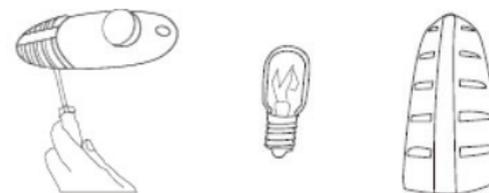
3. Replace with an E14 bulb of MAX 15-watt. Not all bulbs will fit your refrigerator.
