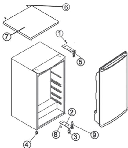
1. Remove the two screws. (6) securing the top. Remove the top (7).
