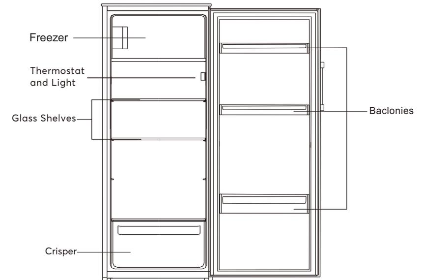
Drawers, food boxes, shelves, etc. placed according to the position in the picture above are the most energy efficient.
