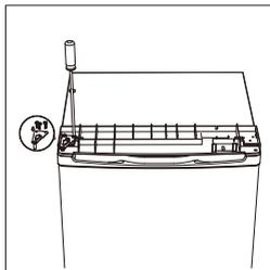
12. Put the top cover and fix it with 2 screws on the back.
