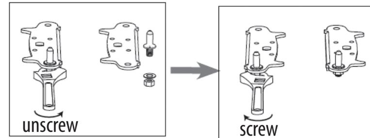
9. Refit the bracket fitting the bottom hinge pin. Replace both adjustable feet. Transfer the lower door to the property position.
