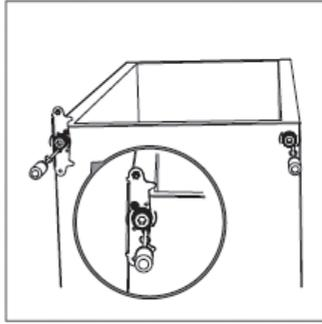
10. Make the middle hinge reverse direction 180°, then transfer it to the left property position. Make the middle hinge pin in the upper hole of the lower door, then tight the bolts.
