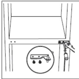
5. Move hinge hole cover in lower door to another side. Then lift lower door and place it on a soft pad to avoid scratch.
