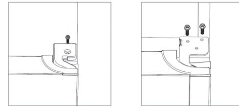
2. Remove the pin with a screw driver and flip the hinge bracket. Then refit the pin to hinge bracket.
