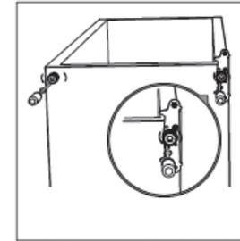
8. Unscrew and remove the bottom hinge pin, replace it by the provided spare bracket and fix it firmly.
