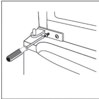
11. Place the upper door back on. Ensure the door is aligned horizontally and vertically so that the seal are closed on all side before finally tightening the top hinge. Then insert the top hinge and screw it to the top of until and then fix hinge cover (in accessory bag) by screw.
