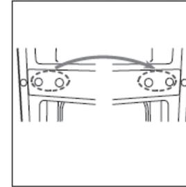
7. Unscrew bottom hinge. Then remove adjustable feet from both sides.
