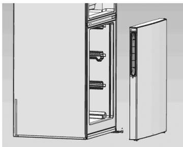
7. Use the tool to take out shaft sleeve in top of refrigerator door and freezer door, put them into the opposite side of door.
