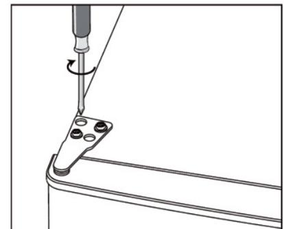
8. Insert the hinge bracket and screw it to the top of the unit.
