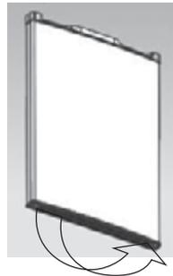
Replace the top-hinge. Replace the door bearing bush and the limit block.
