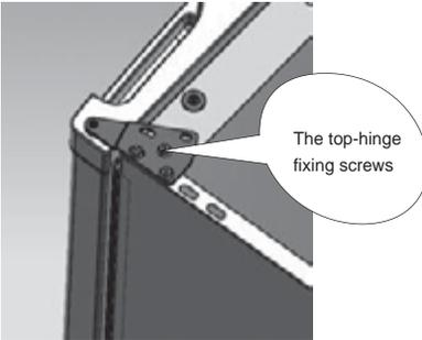
3. Replace the top-hinge and the door limit block and the door bearing bush to the other side.
