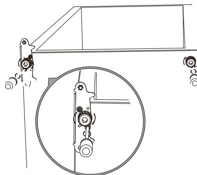
7. Unscrew top hinge pin and mount it to left hole.
