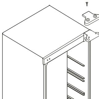
2. Open the door and unscrew the top hinge. Then take the door from the cabinet and place it on a soft pad to avoid damage.
