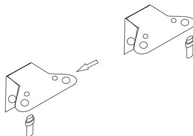
8. Stand up the unit and put the door on the bottom hinge. Make sure the bottom hinge core is inserted in the door hole. Then fit upper hinge with the door. Before tightly fix the upper hinge, try to open the door to check whether the cabinet is sealed well. Finally, screw the hinge cover with hinge.
