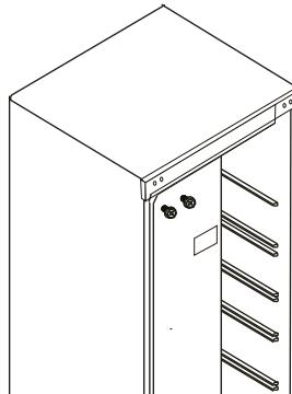
4. Carefully lie down the rear of cabinet on a soft pad. Remove two leveling feet first. Then unscrew the door hinge and left foot base.
